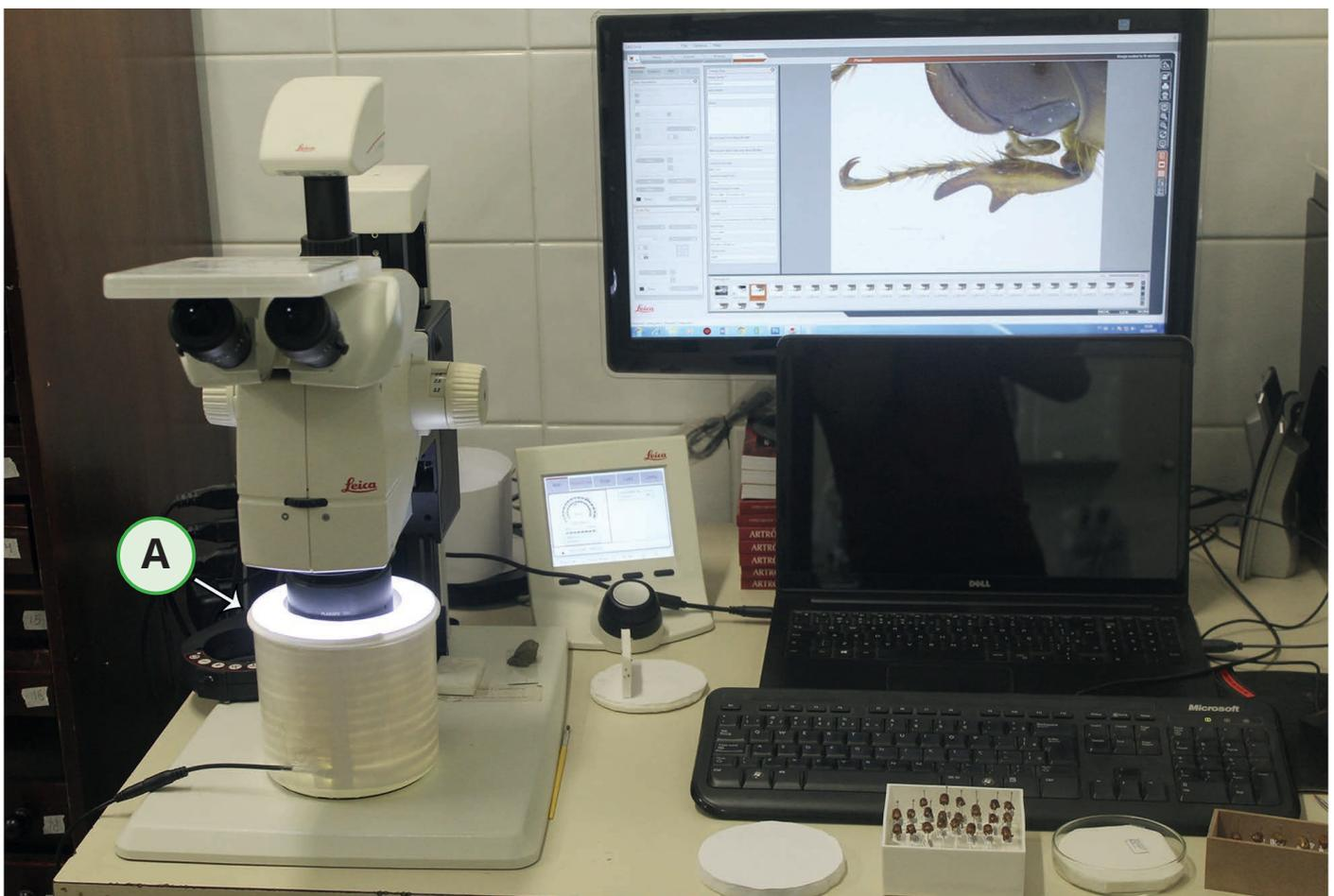
**Figure 3.** Stereomicroscope self-assembly, model Leica M205 C: **A)** circular LED dome lighting system.
